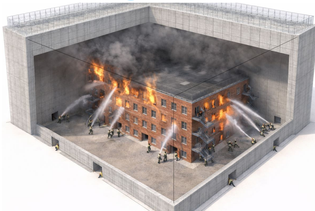
Figure 3 – Visualization of firefighting operations within the space between the protective structure and the facility building
