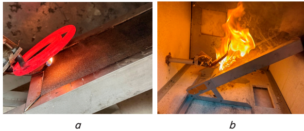
Fig. 10. Test results from determining the flammability index of tent fabric treated with epoxy resin: a – thermal effect on the sample; b – ignition of the sample and flame spread
