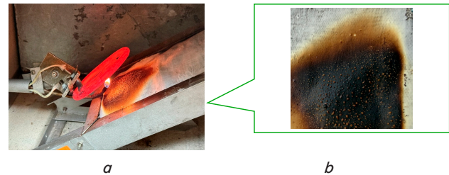
Fig. 11. Test results from the process that determines the flammability index of tent fabric treated with epoxy resin, filled with a mixture of ammonium polyphosphate and aluminum hydroxide: a – thermal effect on the sample; b – ignition of the sample and flame spread
