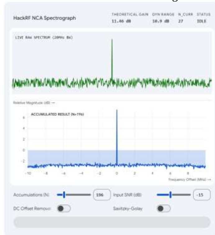
Figure 1 – Amplitude spectrum of the input I/Q signal prior to processing by the NCN algorithm (adapted from data from the SDR system)
