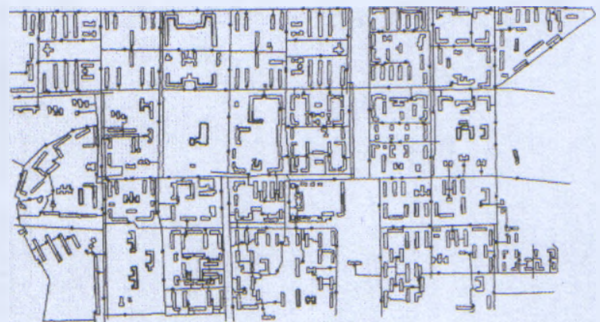
Fig. 6. Placement of fire hydrants (dots on the water supply network) in Ordzhonikidzevskiy area of Kharkov, Ukraine
