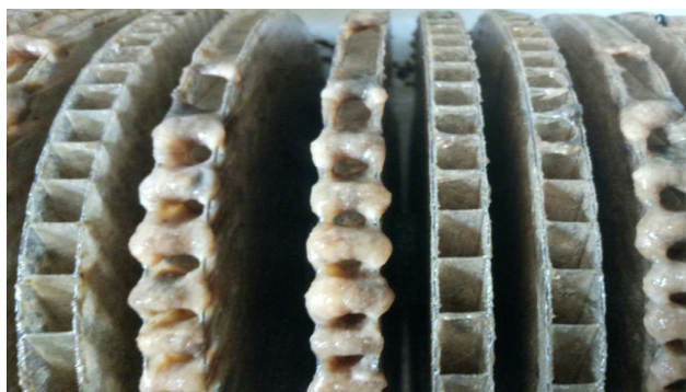
Fig. 2. Bioreactor disks with immobilized biomass
