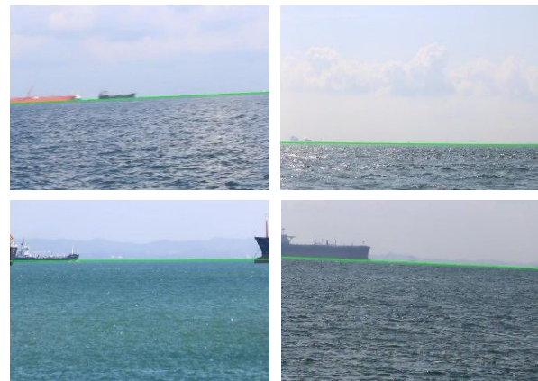
Fig. 11. Some sea-sky line detection result (in green) by proposed method
