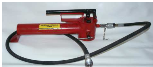
Fig. 2. Hand pumping station HC-35.8
