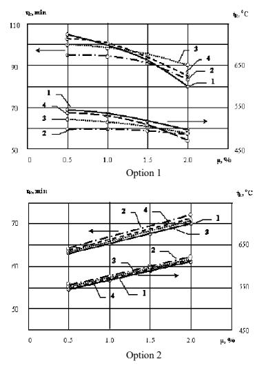
**Figure 1.** Dependences of the critical temperature and fire resistance of bending reinforced concrete elements with fiber reinforcement on the percentage of reinforcement of steel reinforcement when calculated according to option 1 and option 2: 1 – without fiber reinforcement; 2 – steel fiber; 3 – basalt fiber; 4 – synthetic fibers
